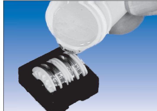
Durapot 864 is Used to Pot an Electronic Assembly to Prevent Vibration Damage
